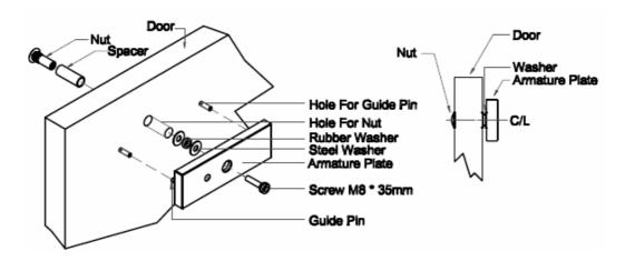
Typical Installation of the electromagnetic lock:
