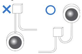
2. Any PoE, power, audio and I/O cables are waterproofed using waterproof silicon rubber or the like.
