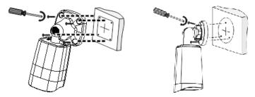
Lead tapping screws through the guide holes in the base and fix them on the wall by using a screwdriver.
