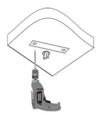
2. Insert the screw anchors.
