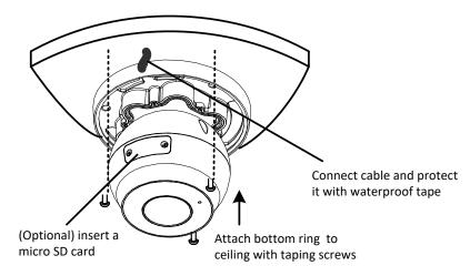
5. Mount the housing by adjusting to the position as shown and press and turn to anywhere but **①**.
