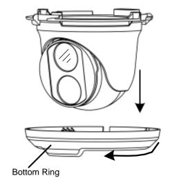
4. Connect the cables and secure the camera.
