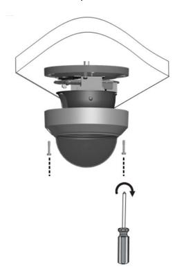
**Note:** Before securing the transparent dome cover, make sure the waterproof rubber strip is tightly held by the six retainers on the bottom ring.
