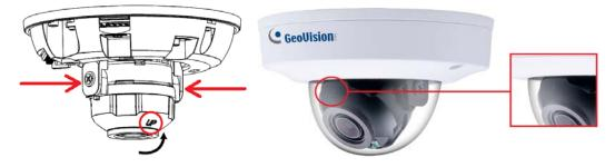
**Note:** Make sure to adjust the lens as stated in Step 4 for any type of installation, in order for the lens to rotate smoothly upon powering up. For installation on the wall, also make sure the "UP" indicator is facing up towards the ceiling.
