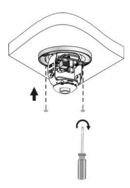
5. Adjust the monitoring direction and tighten the screws after vertically adjusting the lens.
