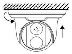
Push the bottom ring back up and turn it clockwise to lock into position
