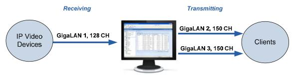
GV-Recording Server + 3 Network Cards assigned on different networks
