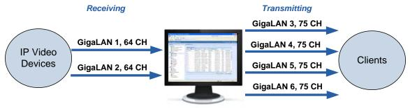
GV-Recording Server + 6 Network Cards assigned on different networks
